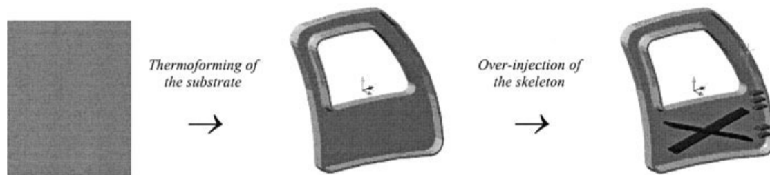
Figure 1 Principle of the new injection-molding/thermoforming hybrid process.
